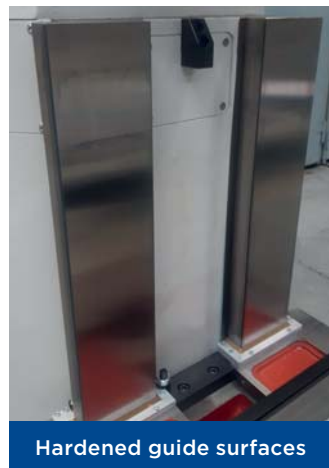
Hardened guide surfaces
